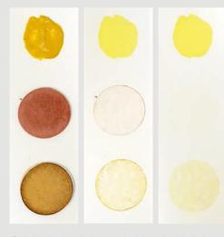
Soiled, wiped and cleaned vinyl-based tablecloth with standard finish.
