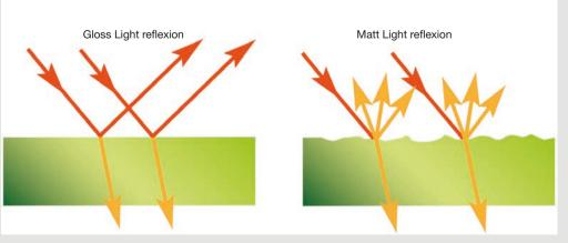
Even high-gloss surfaces (left) reflect the light completely or partially specularly, while uneven surfaces (right) reflect the light diffusely. This causes the observer to perceive the object as matt.
