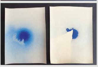
Comparison of standard surfaces (left) and anti-graffiti surfaces (right); the anti-graffiti topcoat ensures easy removal of the graffiti paint by simply wiping it off.
